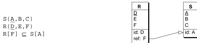
Figure 1: Two representations of the concept of foreign key in the relational model: attribute R.F is a reference to S , a role that is expressed by an inclusion constraint (left) or the tag ref (right).
